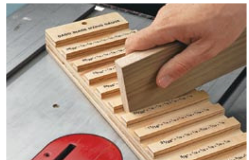
▲ Dado Blade Gauge. This shop-made guide helps determine which parts are needed to make the perfect-sized dado.
