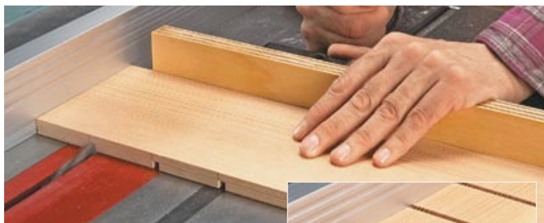
▲ Matched Dadoes. After cutting the dadoes, ripping the workpiece to width provides matched dadoes.
