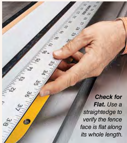
▲ Is it Square? Check the fence face in several places to see that it's square to the saw table.
