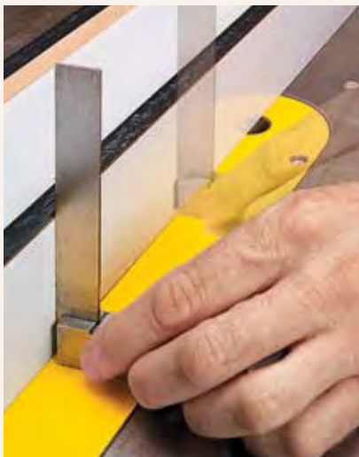
▲ Is it Square? Check the fence face in several places to see that it's square to the saw table.
