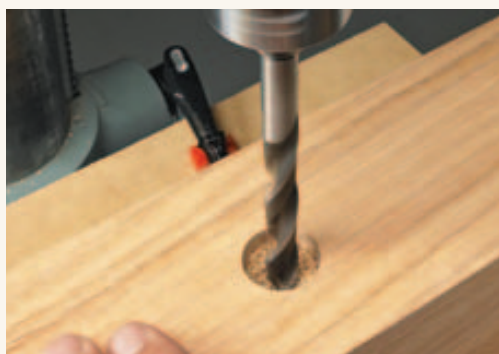
▲ A Counterbored Hole. The drill press makes drilling the counterbored bolt hole in the leg fast and accurate.
