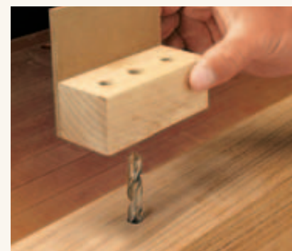
▲ Two Dowel Holes. A drill bit makes it easy to locate the shop-made drilling guide.
