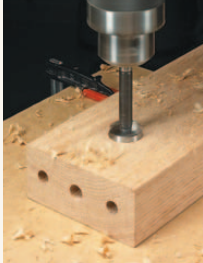
▲ The Cross Hole. Drill the cross hole on the inside face of the stretcher with a Forstner bit.
