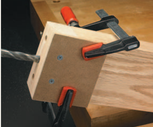
▲ Drilling the Stretcher. A fence on the drilling guide positions the holes properly and allows you to clamp it in place on the stretcher.
