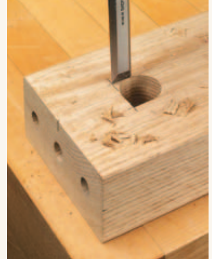
▲ Square it Up. With a chisel, create a flat bearing surface for the washer and nut.
