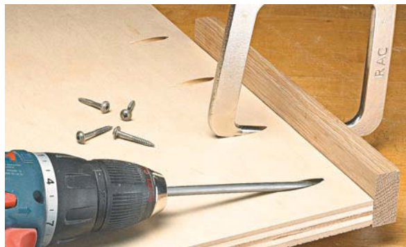
▲ SHELF BANDING Pocket holes are a great way to secure edging to a shelf. A right-angle clamp holds the edging to the shelf while the screws are driven.
