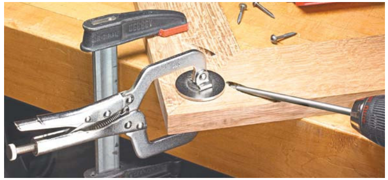
▲ MITER JOINTS Two pocket holes drilled in this small frame secure the miter joint. A face frame clamp makes it easy to hold the joint in position while the screws are inserted.
