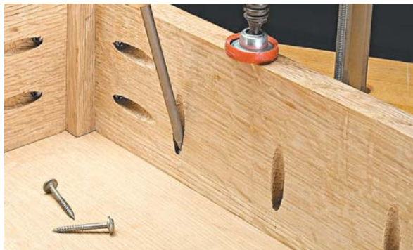
▲ TABLE TOP Pocket holes are perfect for attaching table tops. Drill the pilot hole a bit oversized and back the screw out slightly to allow for wood movement.
