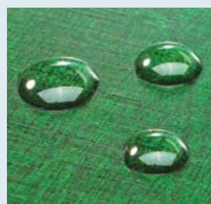
▲ Water-Resistant. A thin phenolic film protects the faces. You’ll want to seal the edges for exterior use.
