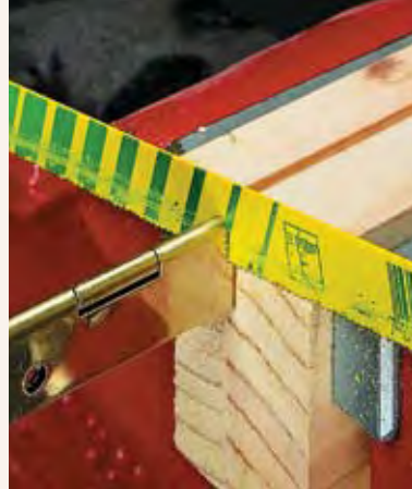
▲ Rabbeted Guide. Clamp a hinge between rabbeted guide blocks for a smooth, straight cut.
