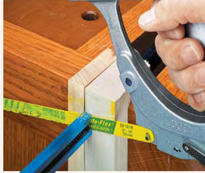
▲ Grooved Support. A dado acts as a support and guide for cutting a section of T-track.
