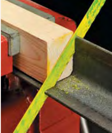
▲ Simple Block. A wood block nestled in angle iron helps guide the blade for a square cut.
