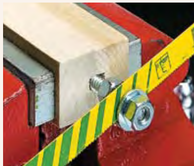
◀ Tube. Insert a dowel to get a cleaner cut and keep the tube from crimping.
